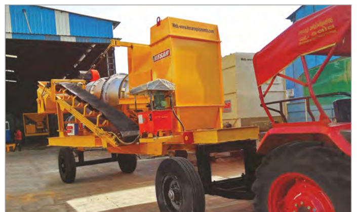
Dryer Drum Unit with Load-out Conveyor
